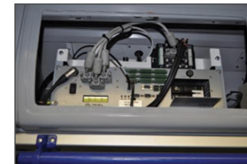
On board recording unit installation
