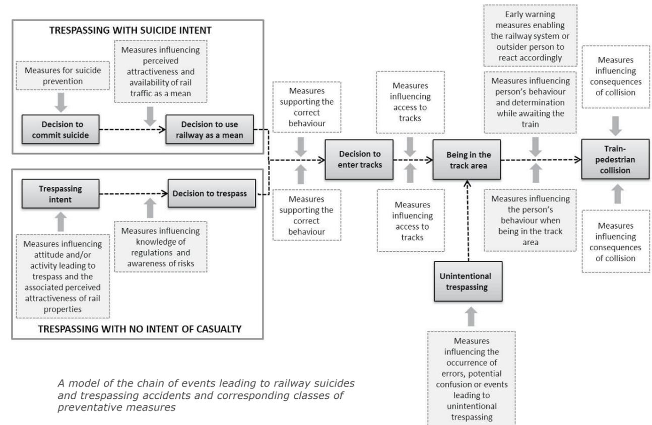
*A model of the chain of events leading to railway suicides and trespassing accidents and corresponding classes of preventative measures*
