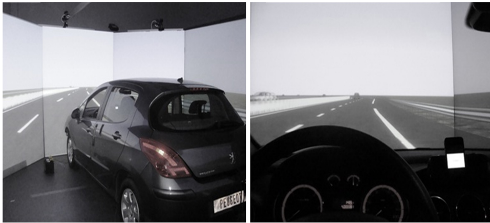
Fig. 1. The Driving Simulator of the Mobility and Behaviour Psychology Lab (IFSTTAR).
